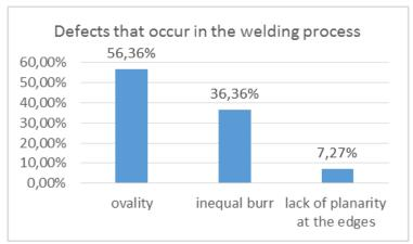
Figure 10. Defects that occur in the welding process
