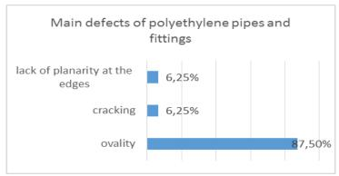
Figure 9. Main defects of polyethylene pipes and fittings
